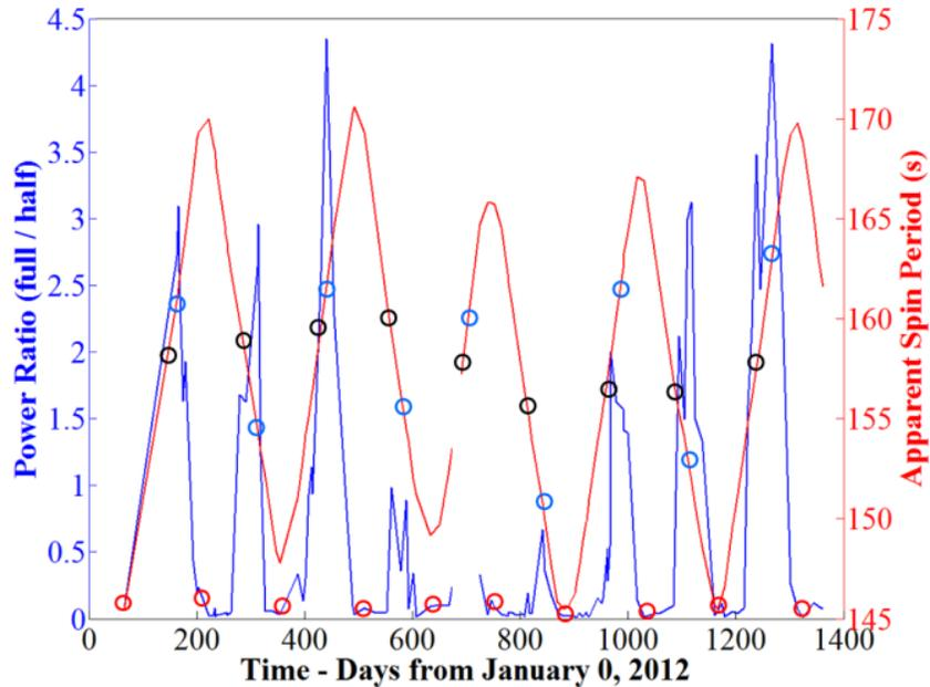
Fig. 5. Telstar-401's full/half period PSR versus spin period
